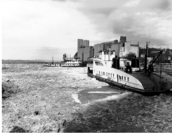
Figure 10-6. Towboats H.L. Frieberg (left) and Dan Lockett (right) breaking ice in the upper lock forebay, Lock and Dam 26, February 1966.
