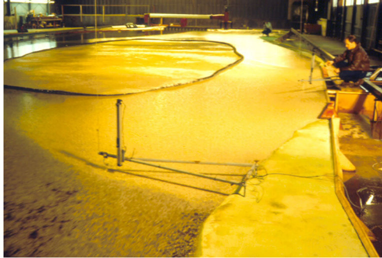
Figure 9-1. Model of Niagara River using crushed polyethylene as model ice.
